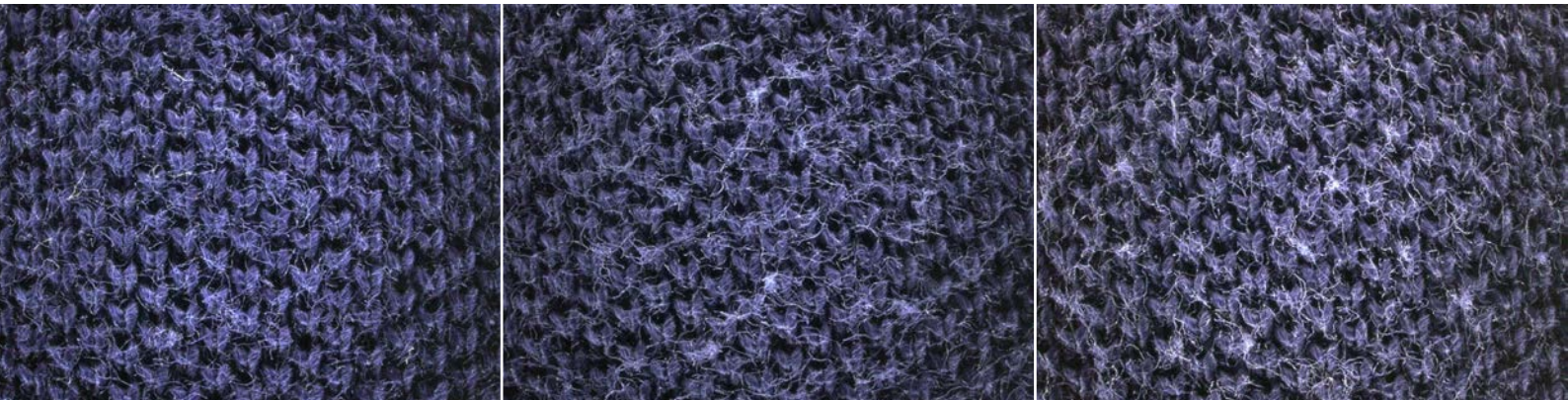
Fig. 1: The pilling test shows significant advantages for the "Rieter" polo shirt made of Com4®jet yarn.
