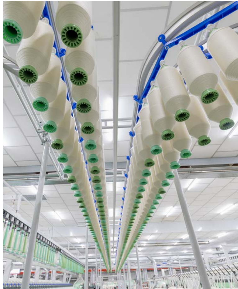
Fig. 6: The roving bobbin transport system SERVOrail enables space-saving and safer interim storage of roving bobbins.
