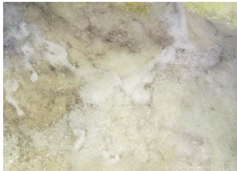
Fig. 2: The sliver feed (top) and the dirt particles (bottom) eliminated during spinning show that the good fibers are fully utilized. The optimized air flow and the improved fiber guidance in the S 36 spin box form the basis for this.
