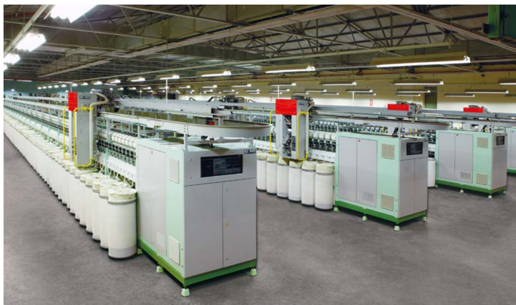
Fig. 6: Spinning mill in Spain with multiple BT 905 machines for processing regenerated fibers
