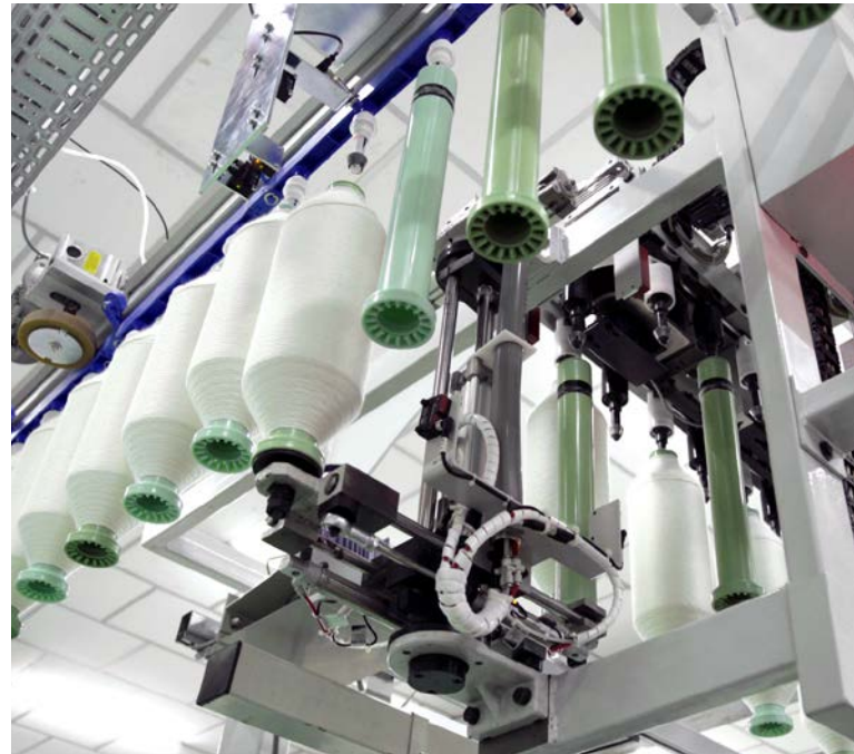
Fig. 3: The bobbin changer can be installed at the head or foot of the machine. This facilitates integration into a transport system.
