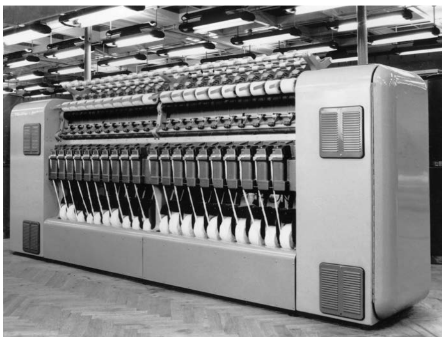
Fig. 1: The world's first model of a rotor spinning machine, in which opening rollers replaced the drafting systems (basis for the M 40-V).
