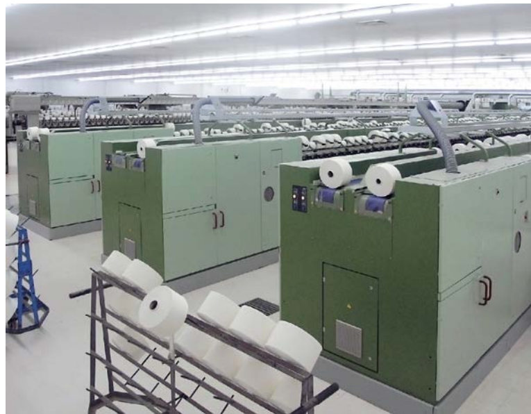
Fig. 7: The BT 923 machine, here in a spinning mill in Thailand, surpassed the magic limit of 100 000 rotor revolutions per minute for the first time in 2005.
