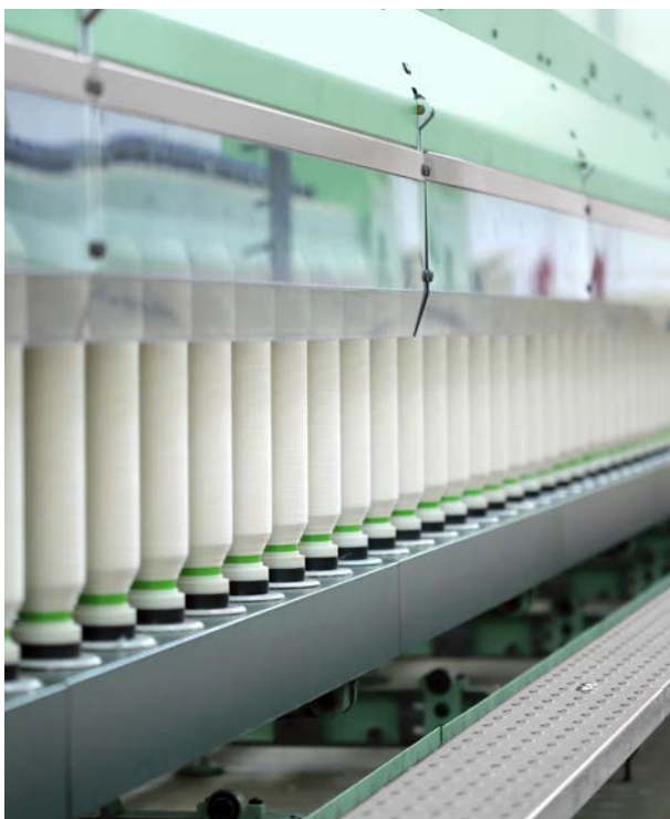
Fig. 2: A long roving frame with 224 spindles supplies three to four ring spinning machines.
