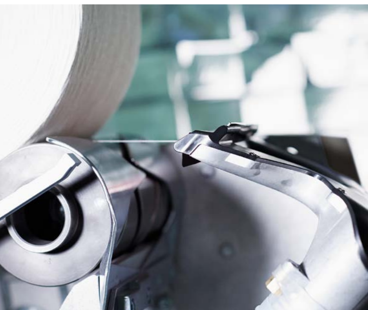
Fig. 1: The optimized suction arm tube enables reliable yarn pick-up when searching for the upper yarn.
