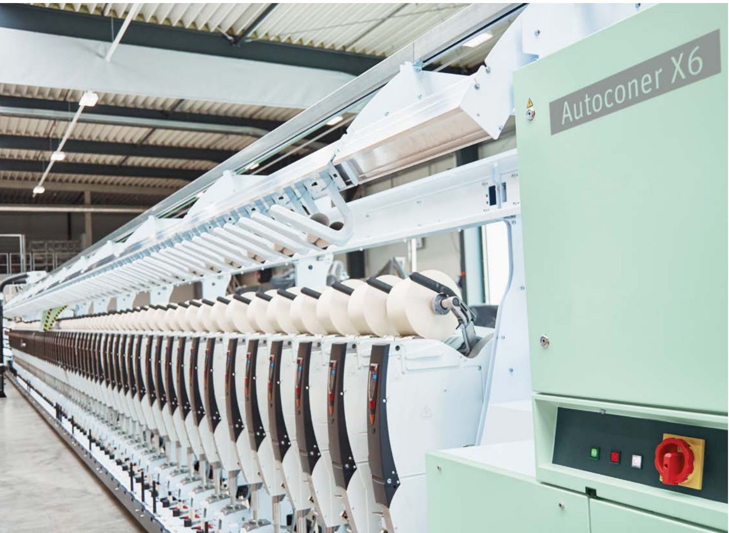
Fig. 1: The Autoconer X6 is the final quality assurance in the ring and compact-spinning process.
