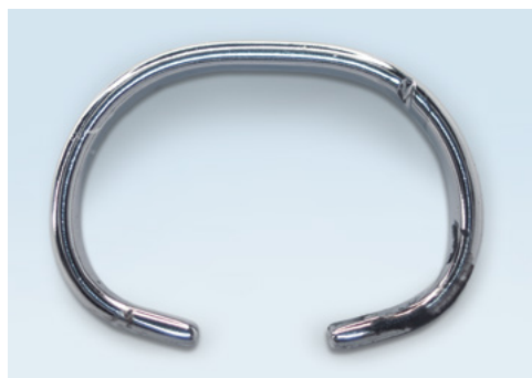
Figure 1: Abrasive wear at yarn/traveller passage
