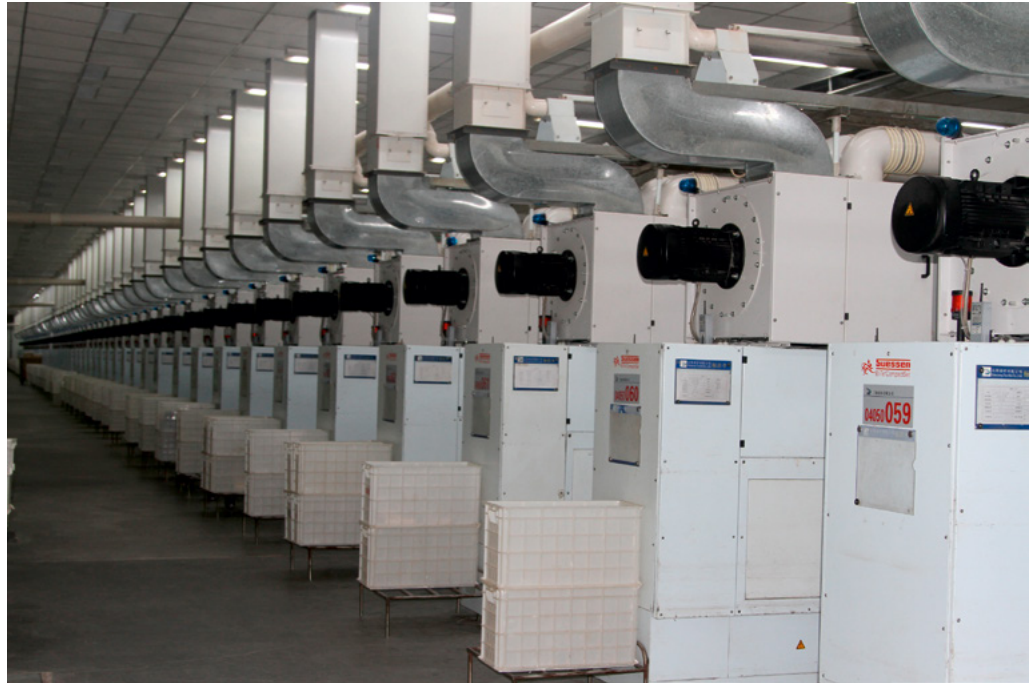
EliTe®CompactSet on Zinser 360 ring spinning frames
