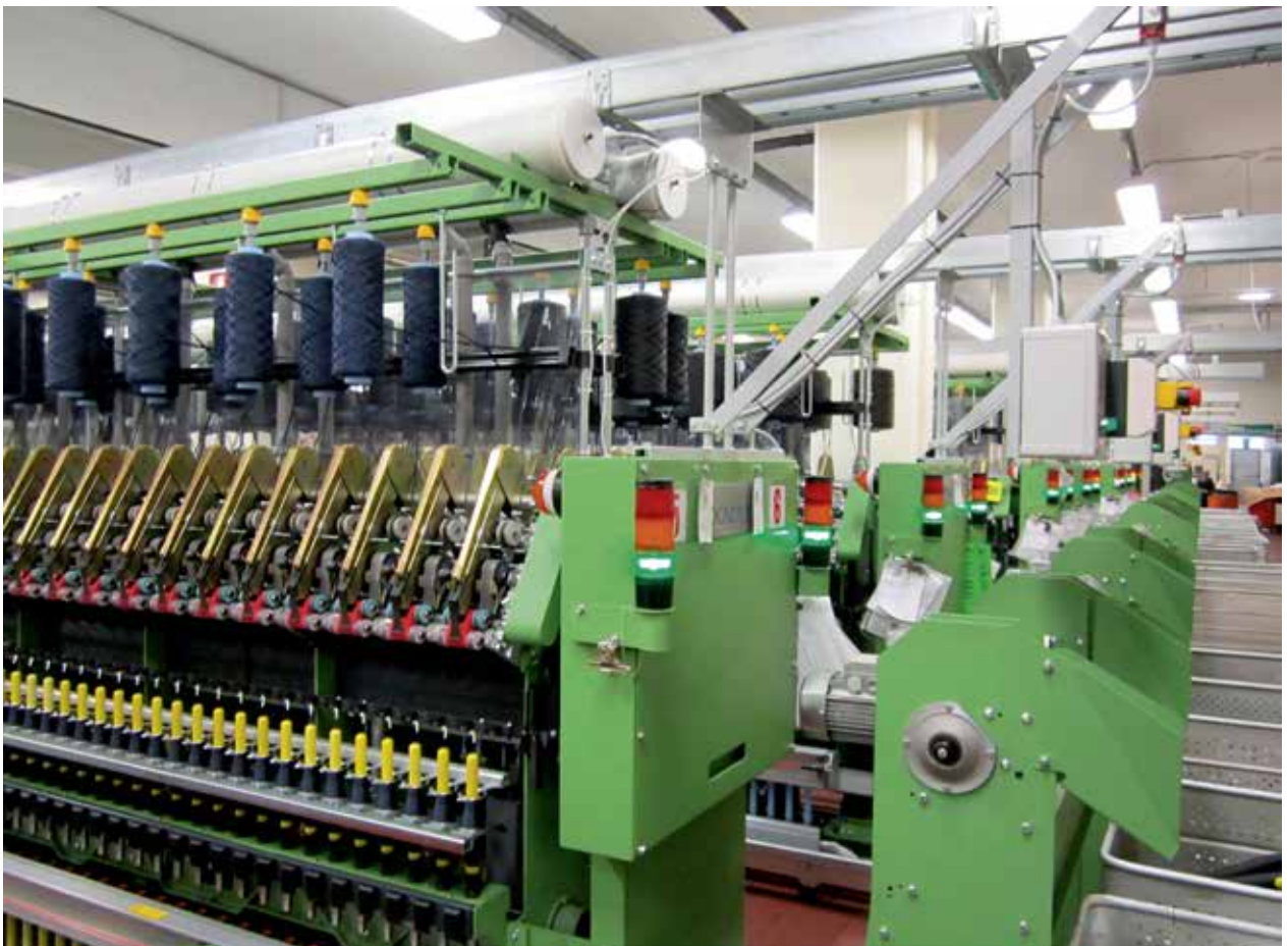
Cognetex IDEA machine equipped with Suessen EliTe® Compact Spinning System
