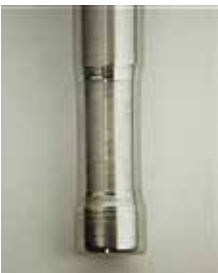
Fig. 5: Worn-out footstep portion of the spindle shaft due to oil contaminated with sand particles
