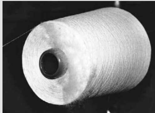
Fig. 13 Fiber fly in knitting accumulated on the package
