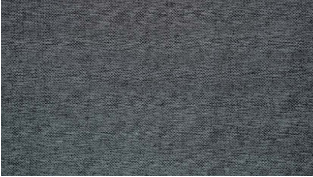
Fig. 14: The black ring yarn fabric shows more nep-like formations.
