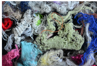
Fig. 2: The degree of fabric opening is decisive for an optimal processing in staple-fiber spinning.
